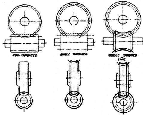
2. A single enveloping (single throated) worm gear is a helical cut and has a parallel-sided gear mating with a curved (concave) worm wheel. This type of gear is more forgiving for position and alignment to tolerance problems. These gears may use ALMASOL Worm Gear Lubricants or the ALMASOL Vari-Purpose Gear Lubricants (consult manufacturers specifications)
