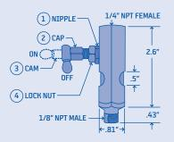
To set or change rate of flow, push cam (3) to horizontal position. Loosen lock nut (4). Turn cap (2) counter clockwise until oil is feeding properly. Lock setting with lock nut (4).
