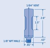
Sights are sized to fit existing or readily available fittings. Heavy duty material is used through (black oxide steel). Sights measure .81" wide by 2.6" high (male) or 2.17" high (female).
