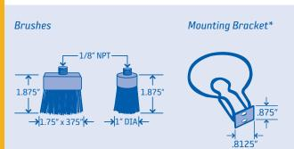
\* Mounting bracket is included with all LubeSite chain oilers or can be used with any of the other oilers. Bracket p.n. 803-7.
