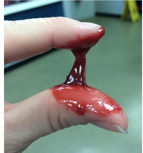
Depending upon the thickener type employed, grease can liquify between 200°F and 500°F (93°C and 260°C). A test that has been used to indicate the liquification point of grease is called the dropping point. As a general rule, the higher the dropping point, the higher the service temperature that can be recommended for a grease. For example, clay-thickened greases are often considered excellent high-temperature greases because they don't have a dropping point.
